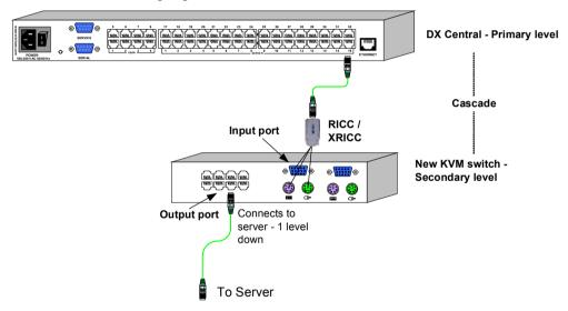
Figure 37 Input and output ports
